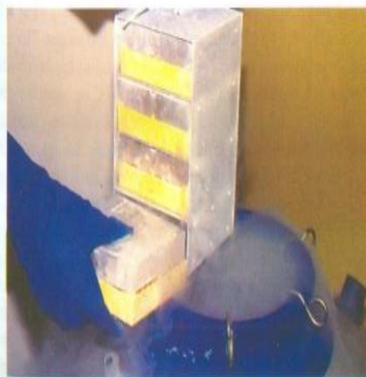
Fig. 6. Liquid nitrogen preservation of cultures
