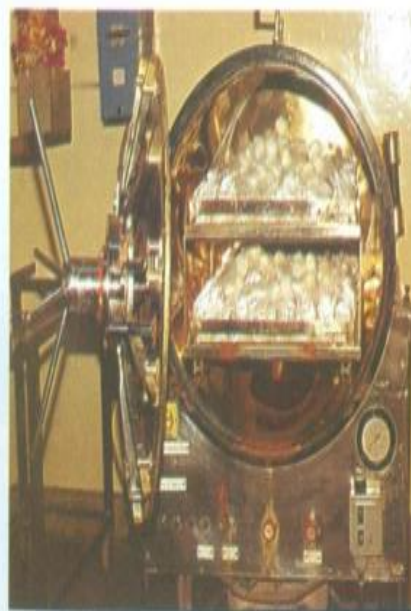
Fig. 10. Horizontal autoclave for sterilization of spawn substrate.
