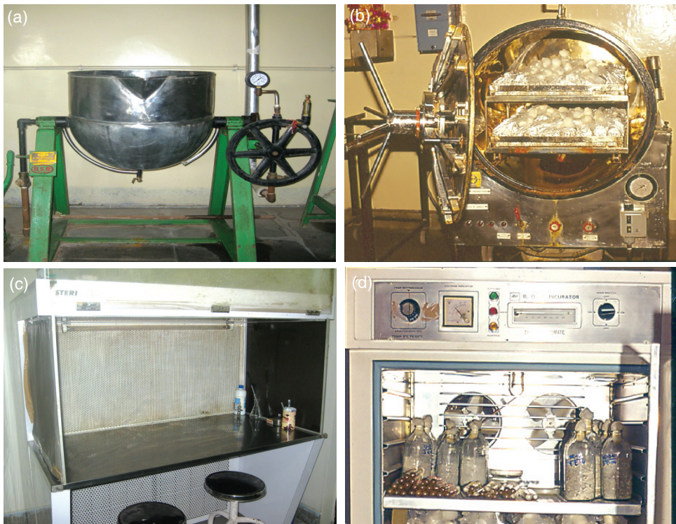
Fig. 5.9. Equipments for spawn laboratory (a) boiling kettle, (b) autoclave, (c) laminar flow and (d) BOD incubator
