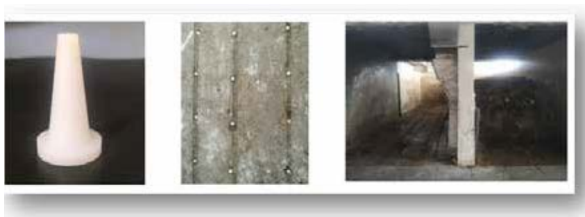
Fig.2.5.11. Nylon plugs for operating large sized phase I bunker for smaller compost lot
