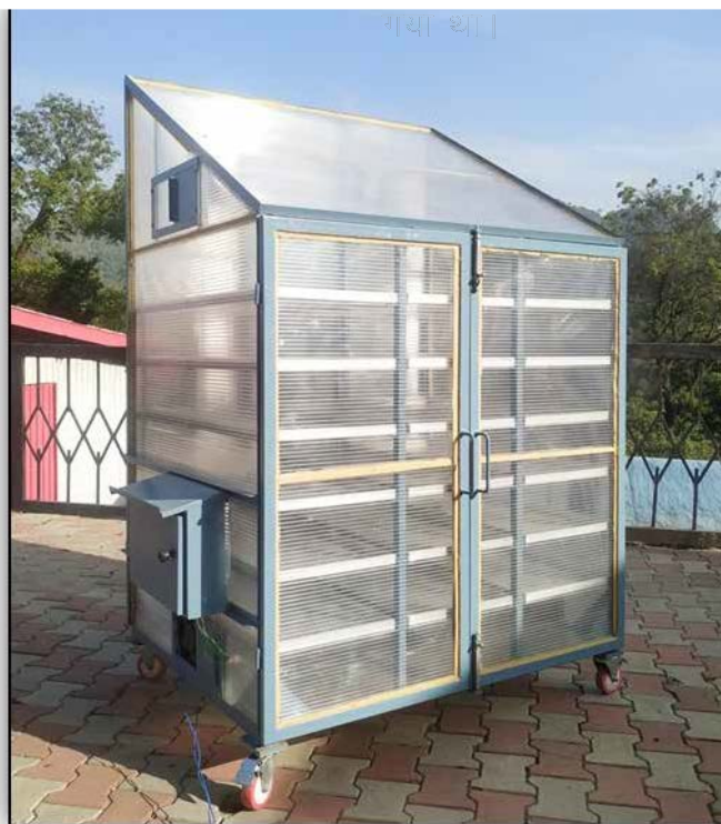
Fig.2.5.8. Modified hybrid solar drying chamber
