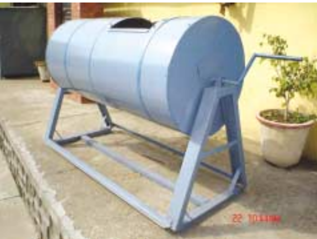
Fig. 2. Substrate mixing drum
