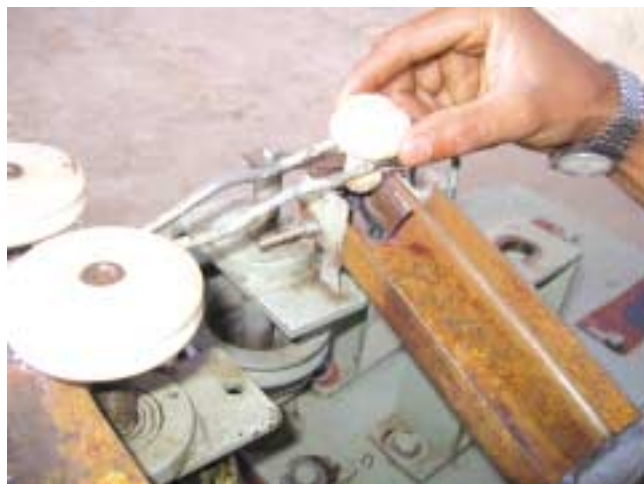
Fig. 4. Close view of mushroom stipe cutting machine during working
