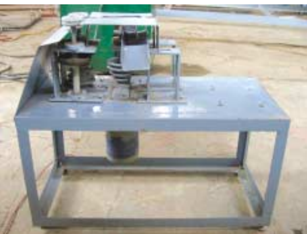
Fig. 3. Front view of mushroom stipe cutting machine
